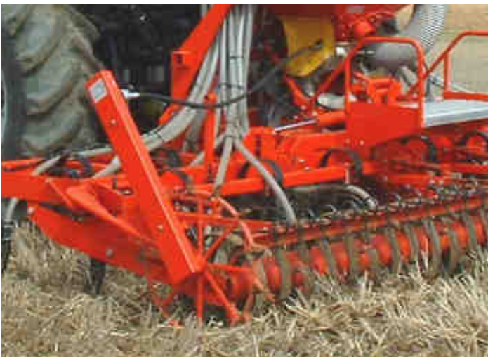
Springflex 400 Roller presses directly over each row
