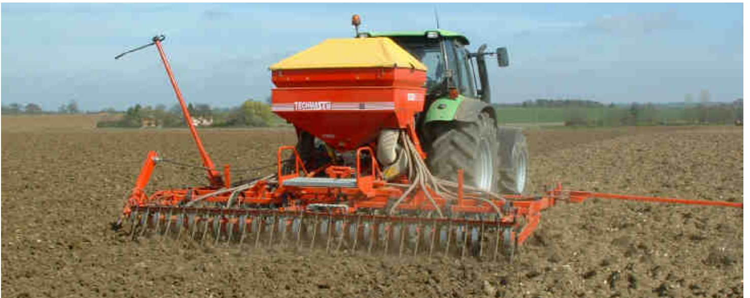
Drilling S Beans direct into ploughed heavy Suffolk clay, minimum depth behind tractor wheels 4", Spring 2007.
