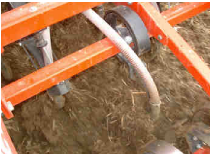
Wide clearance tines can work up to 15 cm deep
