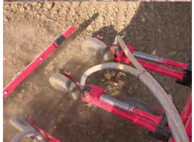
Following harrow sweep tines leave a level finish and do not block in high levels of trash
