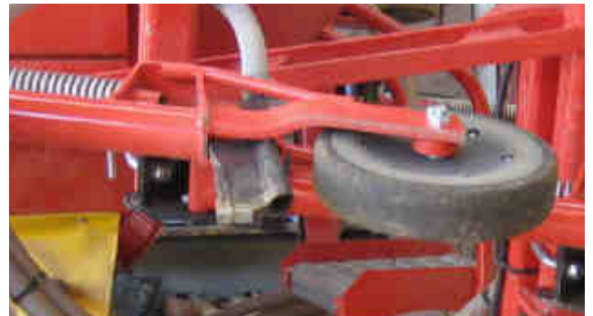
15mm wide Tungsten Carbide coulter tips are designed for long life and can either be straight for tilled ground or forward sloping for direct seeding.
