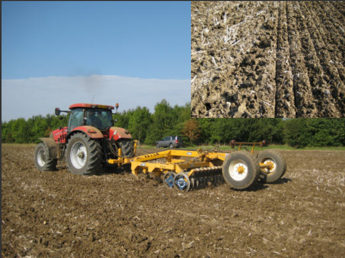
Fields for cereals are pressed, leaving an ideal surface for drilling.
