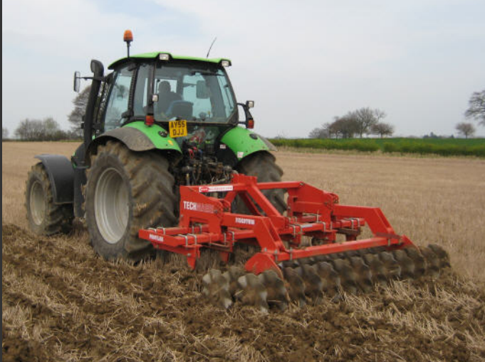
Stubbles are loosened with the Techmagri Profilab when soil moisture is sufficient to deter the creation of clods.
